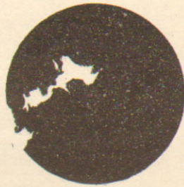
Target showing 5 consecutive shots at 12 1/2 yards, .22 Smith & Wesson pistol, 10 inch barrel, regulation open sights, Peters long rifle cartridges.
