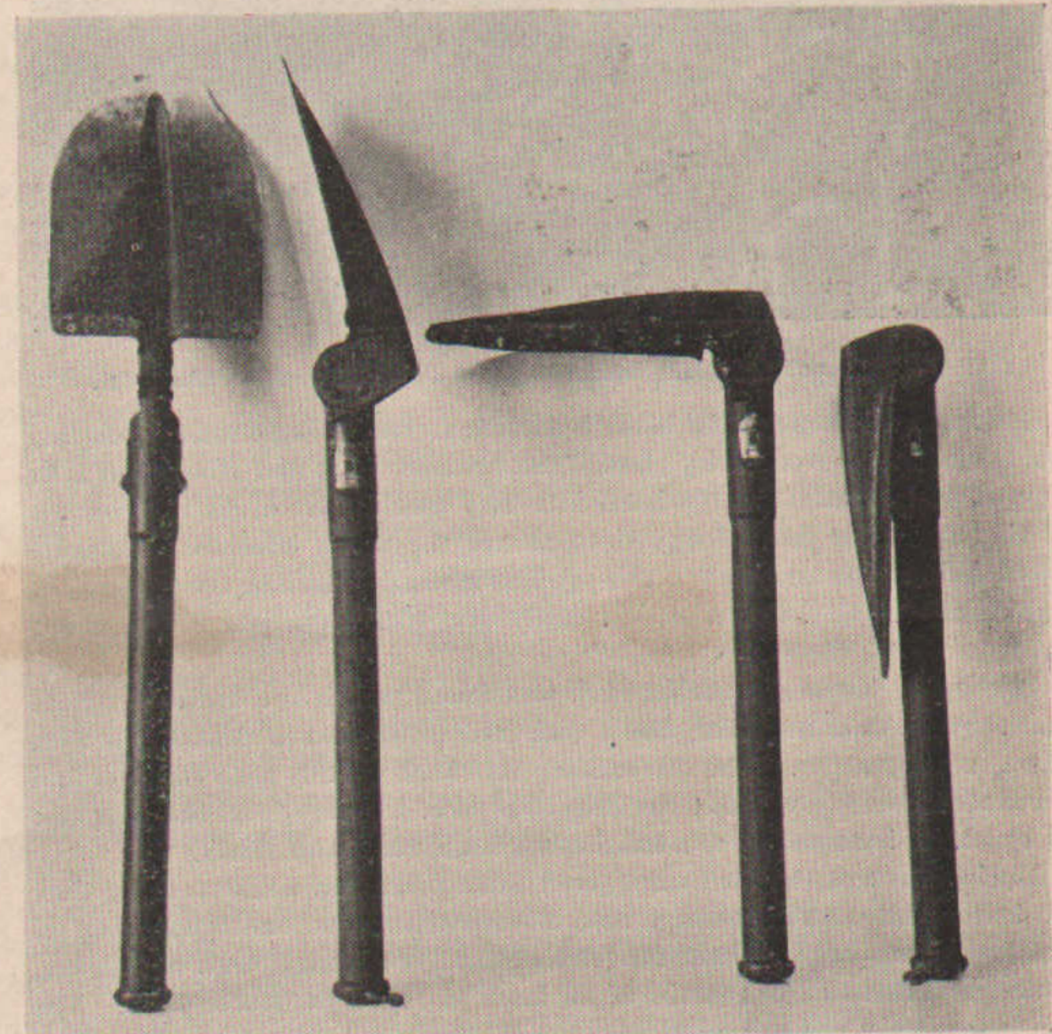
THE ELLIOTT INTRENCHING TOOL IN ITS THREE POSITIONS OF ADJUSTMENT. As a Shovel, Looking at it from the Rear and from the Side, as a Mattock and for Use While Lying Down, folded for Carrying in this Form it can be Slipped Over the Belt and Carried with Comfort Anywhere.
