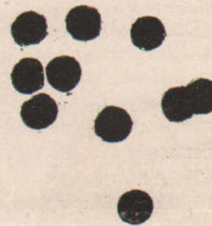
Ten shots at 100 yards from machine rest, by A. O. Niedner, on December 24 with 7½ U. M. C. primer, 21½ grains of Lightning, and 86 grain baseband bullet.
