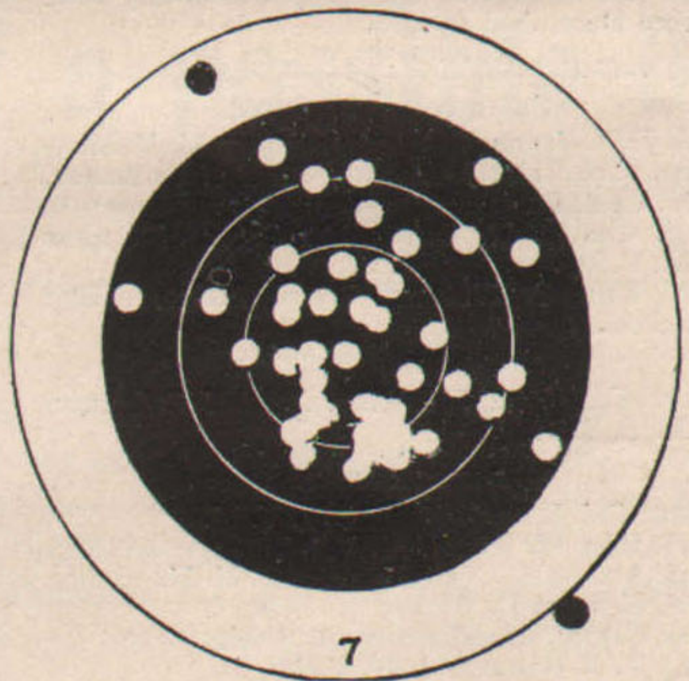
Composite target of winning and record score of 473, made by Geo. Armstrong, of Seattle, Wash., who won the Indoor Pistol Championship, shooting a .22 caliber Smith & Wesson pistol, with 10 inch barrel, and Remington-UMC .22 Lesmok cartridges.
