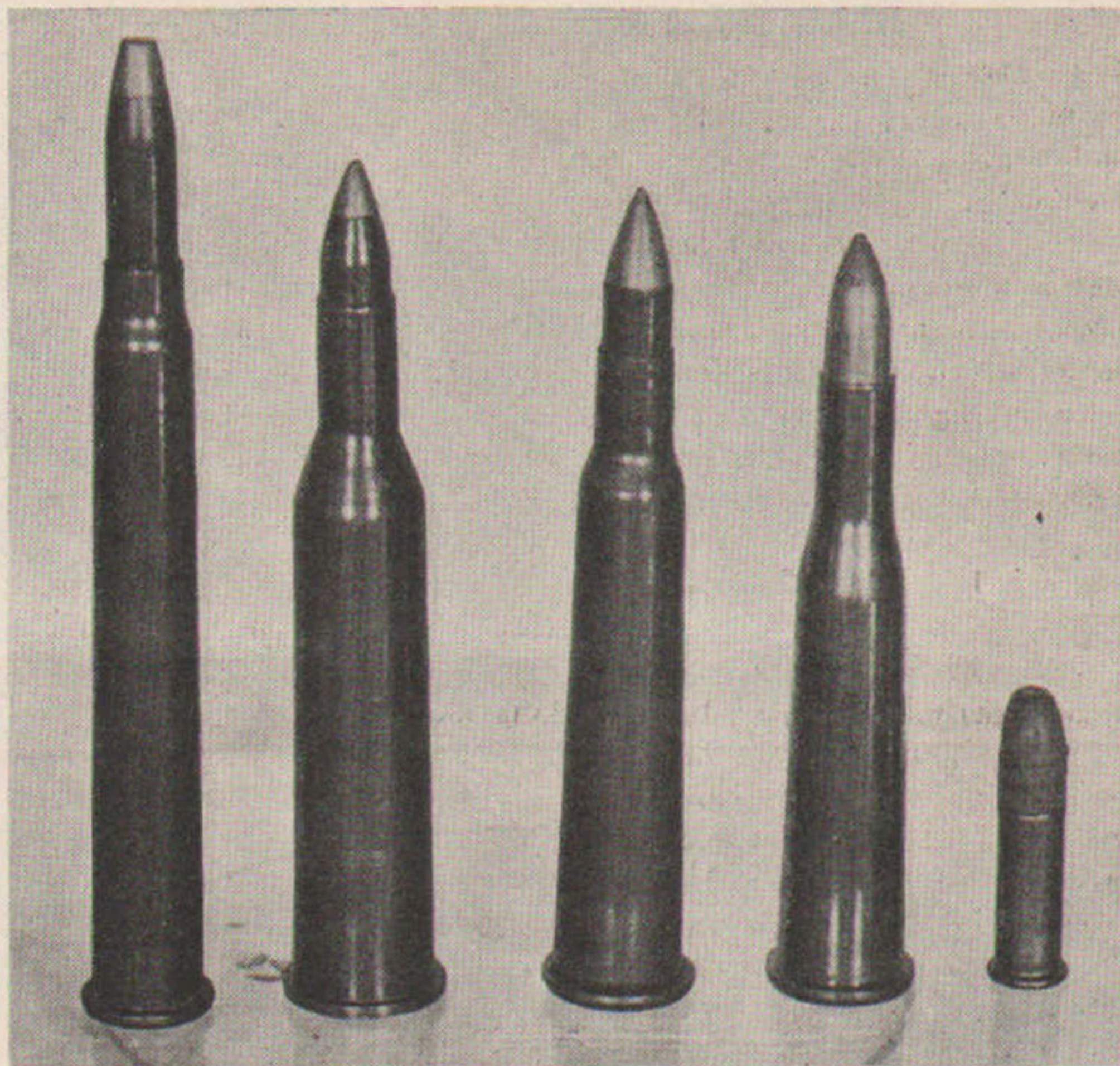
Some .22 Hi-Power Cartridges. Left to right, 28-30 case necked down, Neidner make, Krag case, Knobbe make, 32-40 case necked down Neidner make, Savage .22 Hi-Power: .22 Long Rifle.
