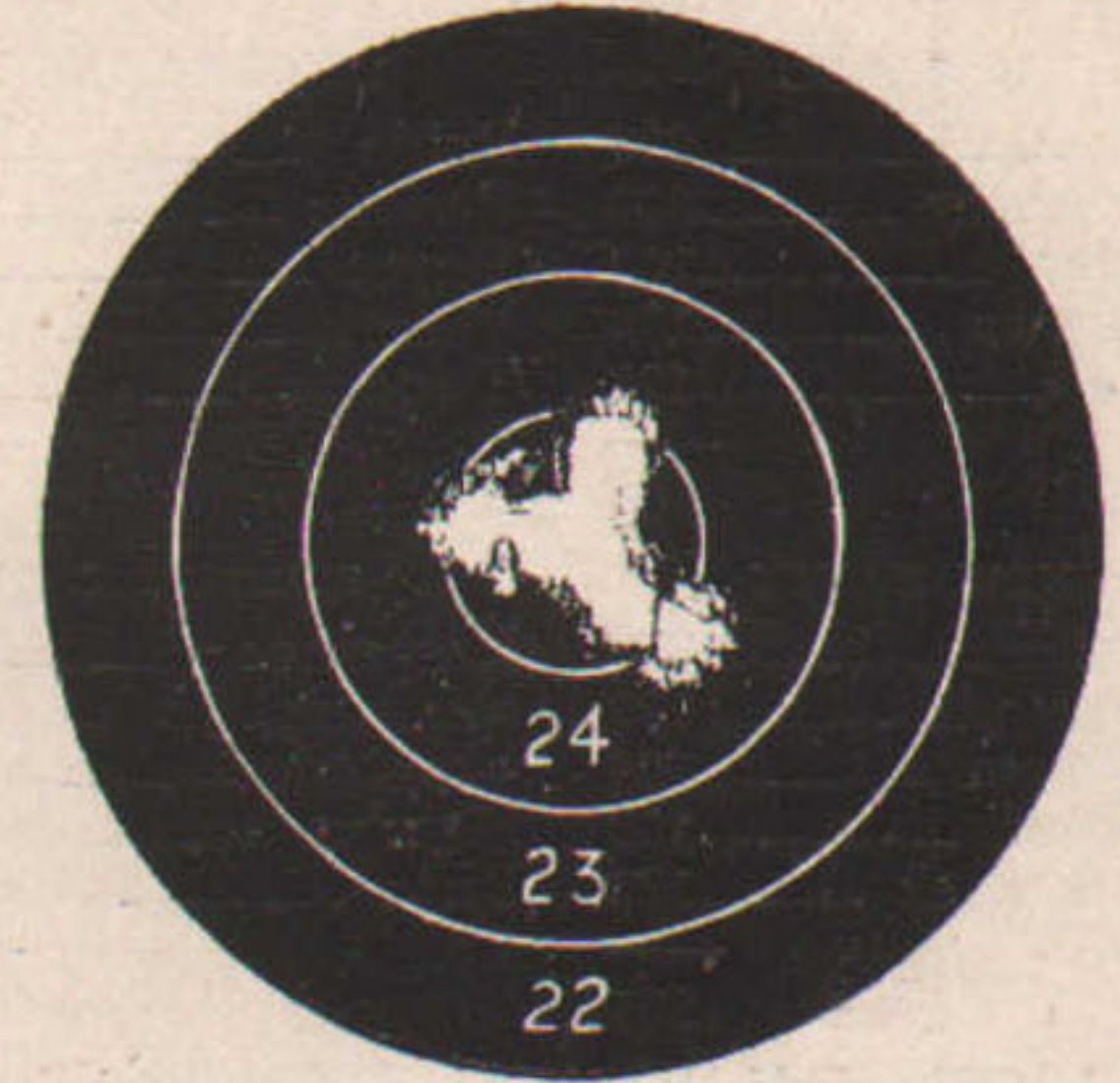
Possible 10 shot score of 250 shot indoors at 75 feet, by H. M. Pope with a Pope-Winchester rifle, Winchester telescope, and Peters .22 shot semi-smokeless cartridges.
