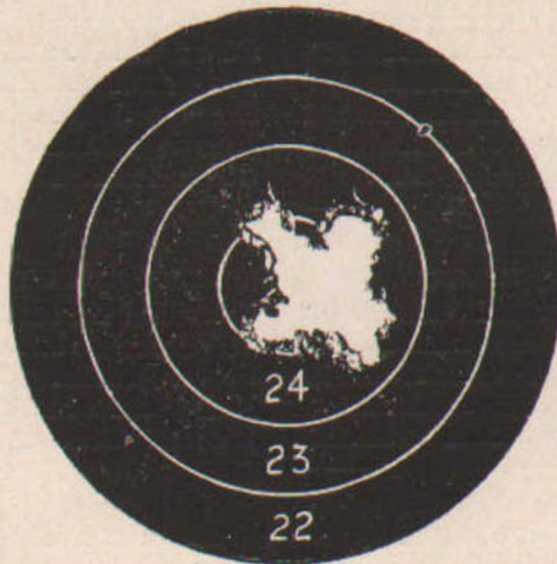
Possible 10 shot score of 250 indoors, by W. A. Tewes at the Zettler Rifle Club gallery, 75-foot range, using Pope-Ballard rifle, Winchester telescope and Peters .22 short semi-smokeless cartridges.
