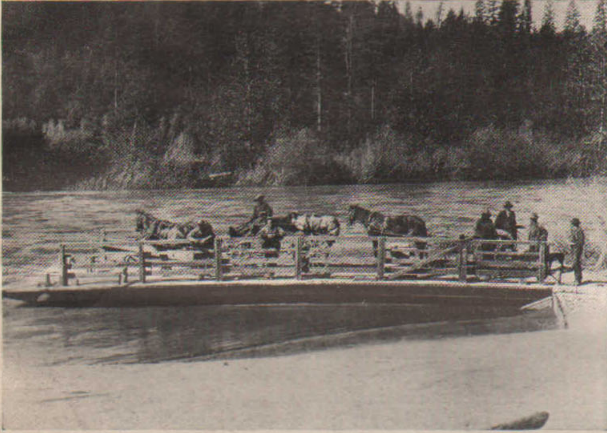
The Way We Crossed Before They Put in the Bridge. The River Kindly Pushes the Boat Across For the Ferryman.
