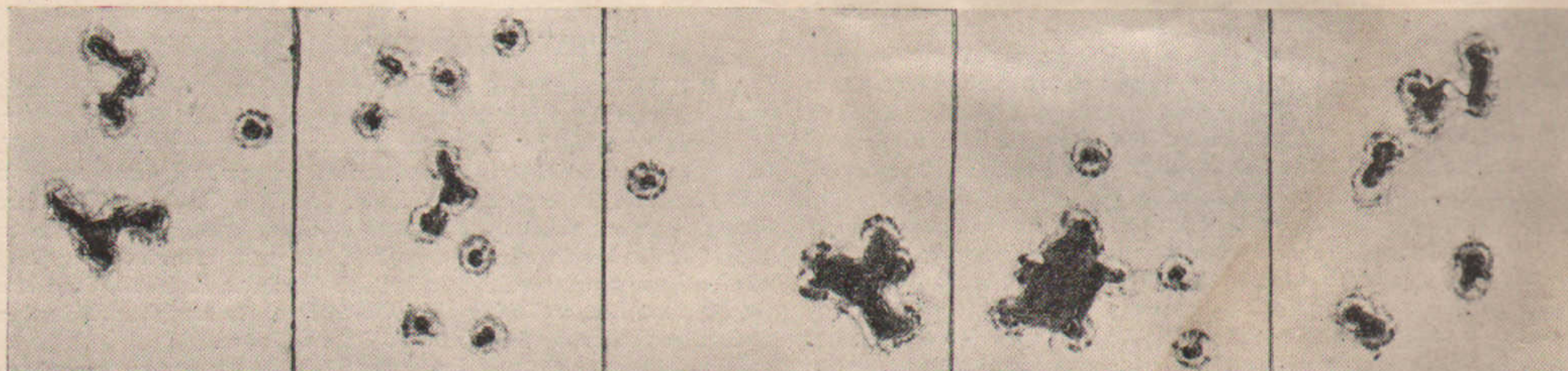
Five 10-shot groups at 100 yards, from machine rest, with Remington-UMC Lesmok .22 long rifle cartridges.
