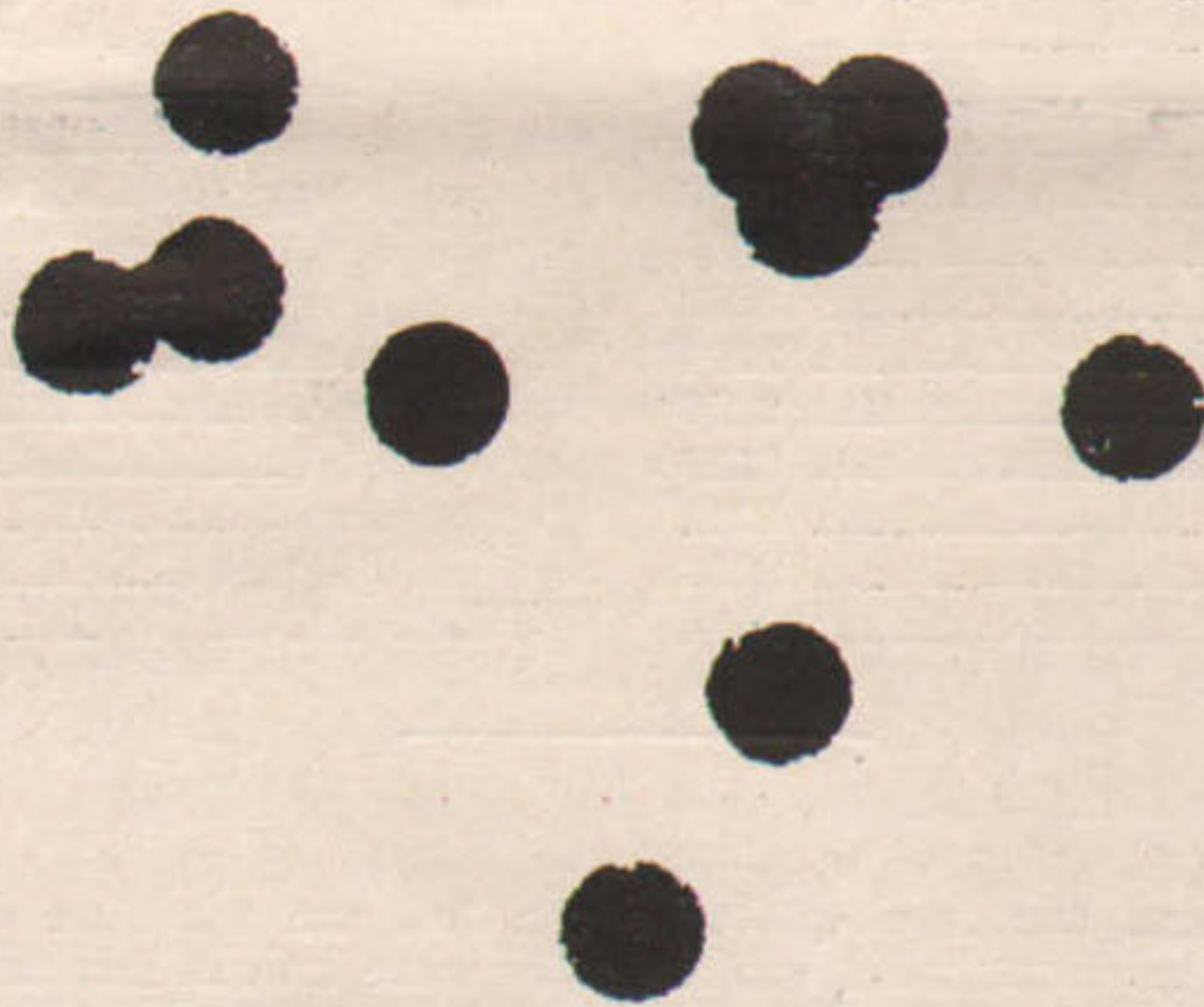
Shot with .38 Schoyen Long Barrel, Hudson Bullet, 1-25; distance, 200 yards, machine rest. Group just a trifle over 2 inches. Shot Dec. 13th, 1912, at 3.30 p. m. Very light 6 o'clock wind. Load: 5 grains bulk K. S. S. F. F. G., 42 grains bulk Schuetzen; Common Primer, U. M. C.; felt wad on powder seated 1/4 inch below mouth of shell. Bullet, 1-25, lubricated with beeswax, tallow and vaseline.
