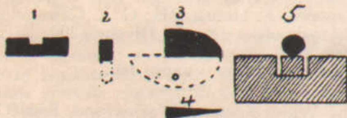
Cut of sights and bullseye (magnified) showing how they should appear to the eye. (1) Rear sight. (2) Front sight as seen by the eye. (3) Front sight side view. (4) Sights and bullseye as they should appear when pistol is properly aimed.
