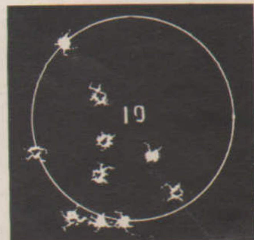
100 Yards—10 Shots, Machine Rest. Group, 1.85"; Mean H. D., .65"; Mean V. D., .55" Mean R. D., .56.
