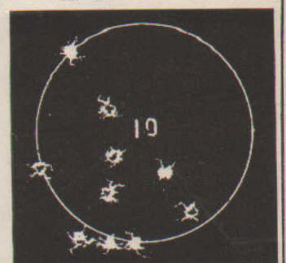
100 Yards—10 Shots, Machine Rest. Group, 1.85"; Mean H. D., .65"; Mean V. D., .55" Mean R. D., .56.
