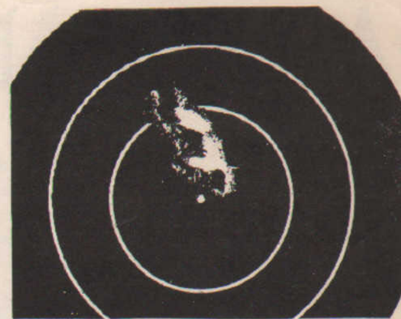
Group made at 20 yards with S. & W. Olympic barrel, no screen. All shots cut a circle 3-8 inches in diameter.
