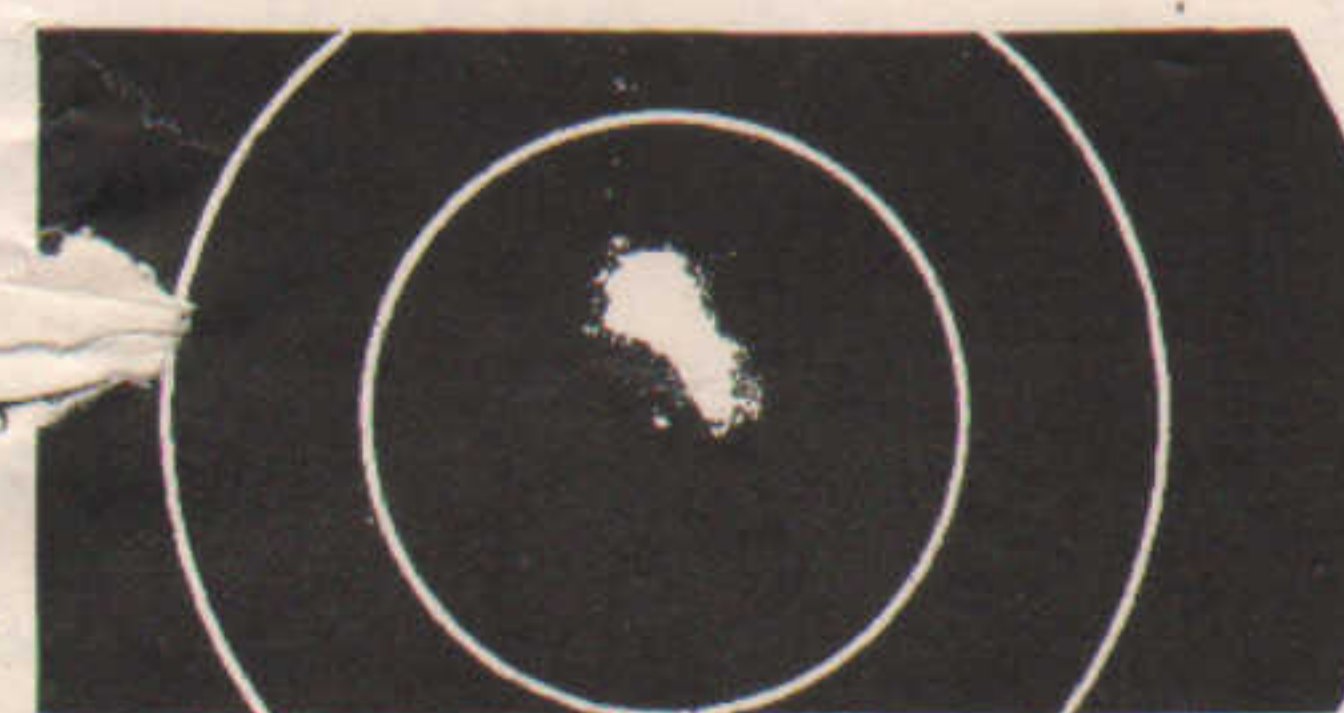
Group made at 10 yards with S. & W. Olympic barrel. Shots will cut circle 1-16-inch in diameter.
