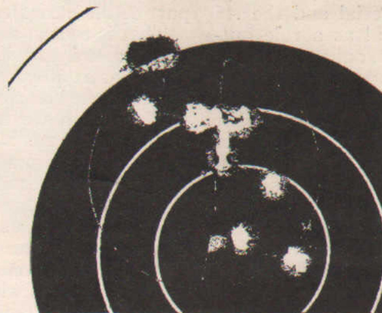
Group made at 50 yards with S. & W. Olympic barrel through 6 screens and two targets. This shows how a group is enlarged by passing through several thicknesses of paper. All shots in 1½-inch circle.
