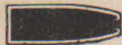
Sectional View Copper jacketed bullet used in Hi-Speed Mush- room cartridges
