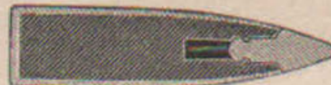
Sectional View Bronze point bullet used in Hi-Speed Bronze Point cartridges (Mush- room)
