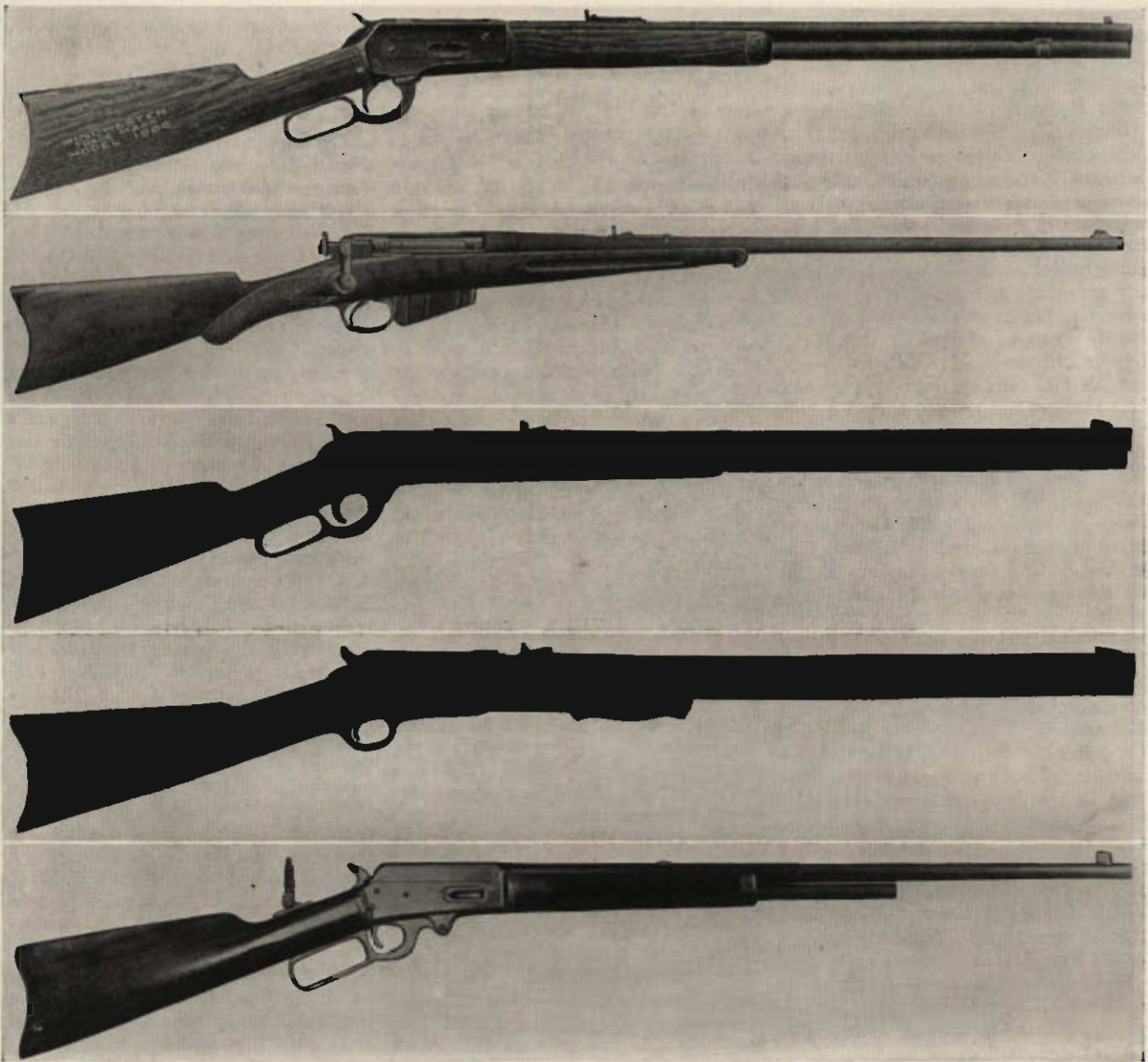
TOP TO BOTTOM: AUTHOR'S WINCHESTER MODEL 1886 RIFLE, .40-45 CALIBER, USED IN THE HUDSON'S BAY COUNTRY 1889-90; REMINGTON-LEE RIFLE, .32 SPECIAL CALIBER; COLT REPEATING RIFLE, .44-40 CALIBER; COLT "LIGHTNING" MAGAZINE RIFLE, .38-56 CALIBER; AUTHOR'S MARLIN MODEL 1893 RIFLE, .25-36 CALIBER
