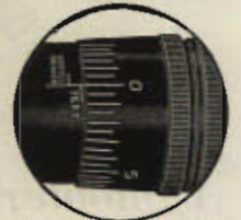
Non-rotating objective lens on front end is adjusted for distance and parallax elimination by graduated sleeve.
