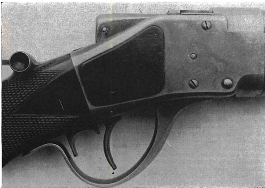
Sharps-Borchardt Single Shot Action with Walnut Side Panels in Receiver. The Safety is located back of the trigger. Receiver of this rifle is beautifully case-hardened and Heat Treated.
