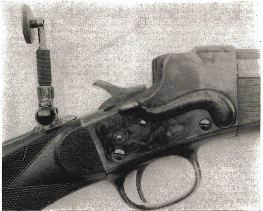
Remington-Hepburn Single Shot Action with Single Trigger and original Side Lever. Action is case-hardened in beautiful colors.
